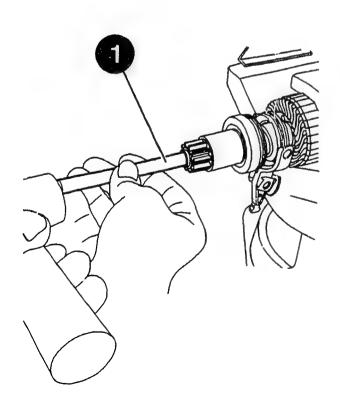
Disassembling overrunning-clutch drive
